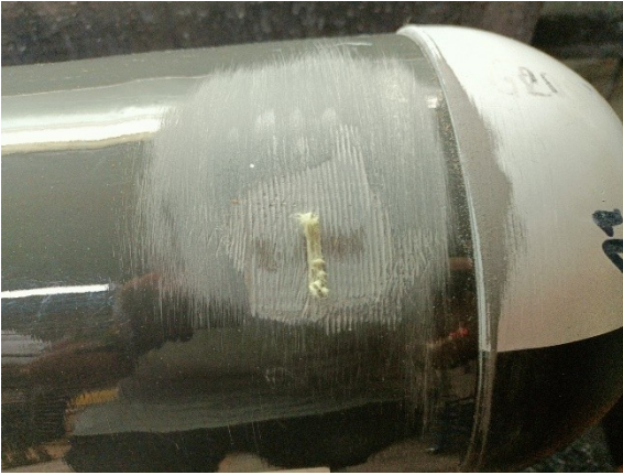
Exemplary damage of level 3 caused by abrasion or cut
