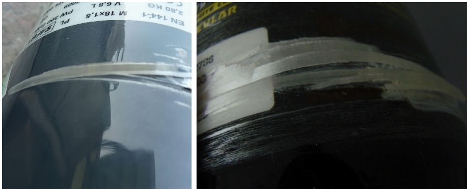
Exemplary damage of level 2 caused by outer shell fibre delamination
