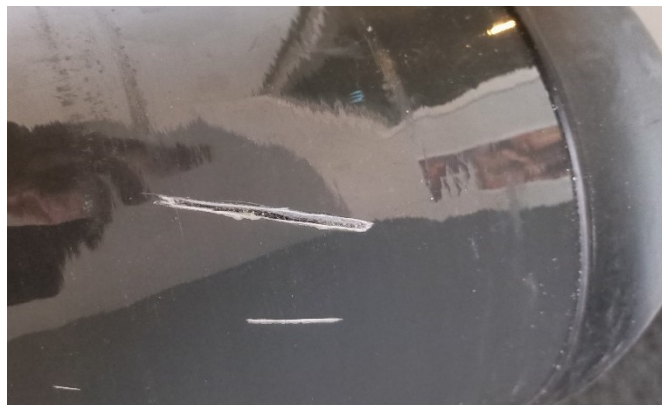
Exemplary damage of level 2 (cut)
