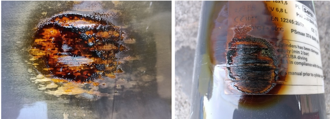
Exemplary damage of level 3 caused by high temperature or fire
