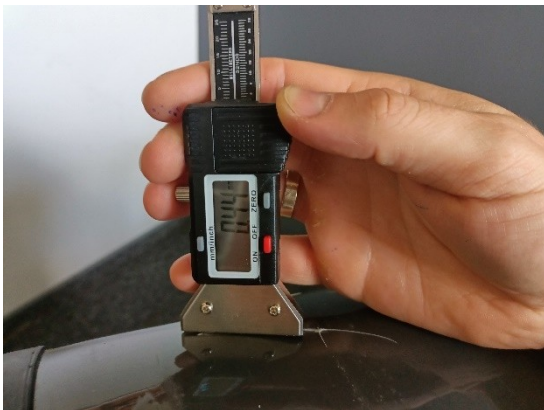
Damage depth measuring method
