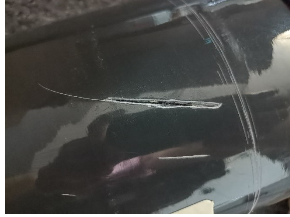
Exemplary damage of level 3 caused by abrasion or cut
