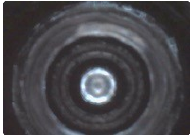
Cylinder interior after filling to 5 bar
