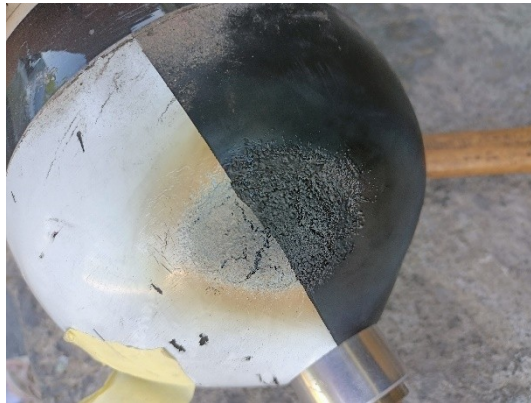
Thermal damage of the rubber shell not affecting the cylinder structure
